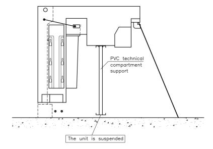
• Make a trench at the base of the technical compartment support. Anchor the base of the support with a length of reinforcement rod (length: 1'). Fill in the hole with mortar (this operation can be carried out when the struts of the swimming pool structure are poured).
