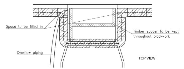
NOTE: the front portion of the overflow piping shall also be embedded in concrete.
